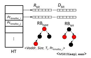
e.g., mov %ecx, (%ebx)  $\rightarrow$  resolve the vaddr of ebx, locate the syscall context by using kernel esp.
